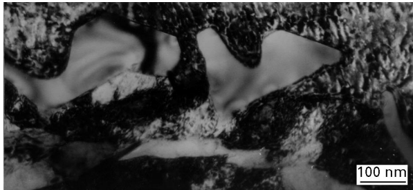
Figure 4 Chromium carbides observed by TEM – 2 at % Mo alloy.
